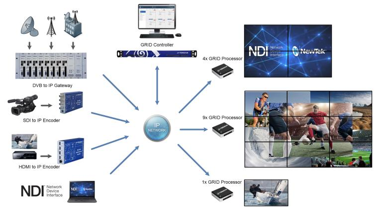
In addition, Teracue's iCue Recording & Media server will add live stream recording and on-demand streaming or scheduled playout. Adding Teracue's MC-ROUTE IP Video matrix to the ICUE-GRID will enable the quick ingest of live streams from network cameras or the Internet in almost any format.
