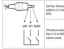
Each Up / Down pin is pulled to 3.3 V with CPU
