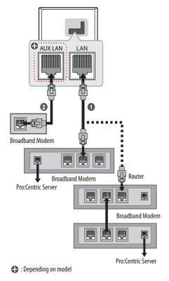
**1** Connect the LAN port of the Modem or Router to the LAN port on the TV.
