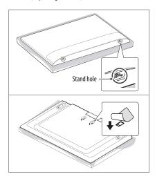
Screw length from outer surface of back cover should be under 8 mm. (Only 24/28LU340\*)
