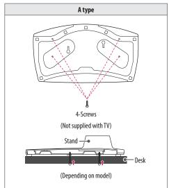
Screw: M5 x L (\*L: Table depth + 8~10 mm)
