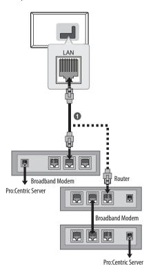
Connect the LAN port of the Modem or Router to the LAN port on the TV.
